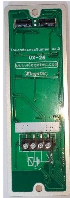
5. Attach the PCB with capacitance sensor pads and LED's
